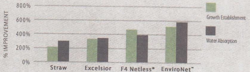
Average values of industry leading single-net straw and excelsior blankets as detailed in public AASHTO-NTPEP reports and independent laboratory testing using standard test methods ASTM D1117 and D7322.
